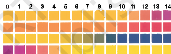
Fig. 6.11 pH-paper with four strips that may have different colours at the same pH
