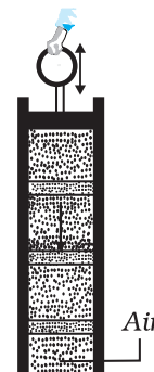
Fig. 14.4 Longitudinal waves (sound) generated in a pipe filled with air by moving the piston up and down. A volume element of air oscillates in the direction parallel to the direction of wave propagation.
